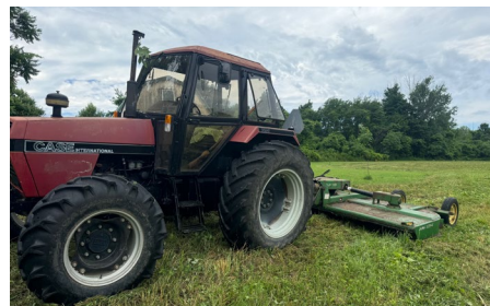
An enclosed cab is a safer option to protect against sap exposure while mowing.
