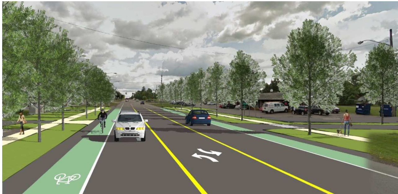
Photo simulation (left) showing restriping Main Street with bike lanes, addition of street trees and removal of excess asphalt along frontage compared to existing (below) and the visual impact it can make on the corridor.
